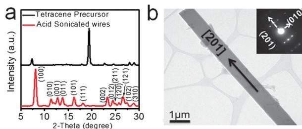
**Fig. 3** (a) XRD patterns of the tetracene crystal and nitric acid-sonicated sample. (b) TEM image of a single nitric acid-sonicated wire. The upper-right inset shows its SAED pattern.
