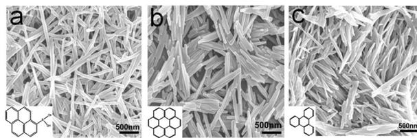
**Fig. 5** SEM images of nitric acid-sonicated (a) 1-pyrenylboronic acid nanorods; (b) coronene nanorods and (c) triphenylene nanorods.
