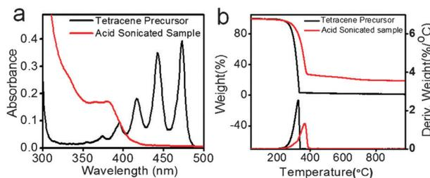
**Fig. 4** (a) UV-vis absorption spectra of THF solutions of the tetracene and nitric acid sonicated sample. (b) TGA weight loss curves (upper) and derivative curves (below) of the tetracene and acid-sonicated sample.
