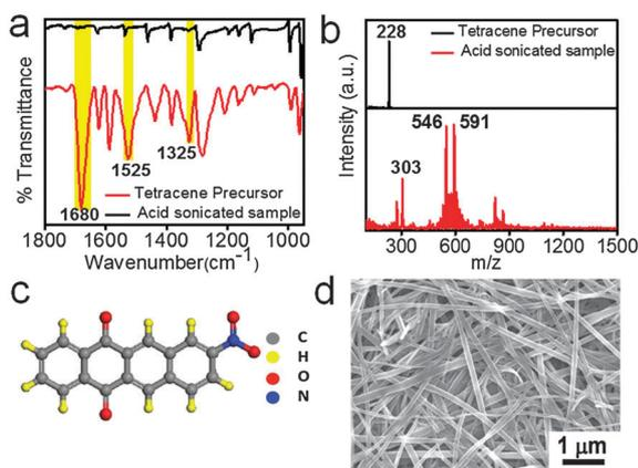
**Fig. 2** (a) FTIR and (b) MALDI-TOF MS spectra of the starting tetracene and nitric acid sonicated nanowires. (c) Proposed structure corresponding to  $m/z = 303$  peak. (d) SEM images showing a network of nitric acid-sonicated nanowires.
